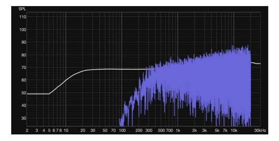
As can be seen from this chart (most of the peaks in this test happened to be in the higher end of the scale) Which means overall headroom can be as high as 90dB, without the hassle of causing noise pollution outside of the venue.
